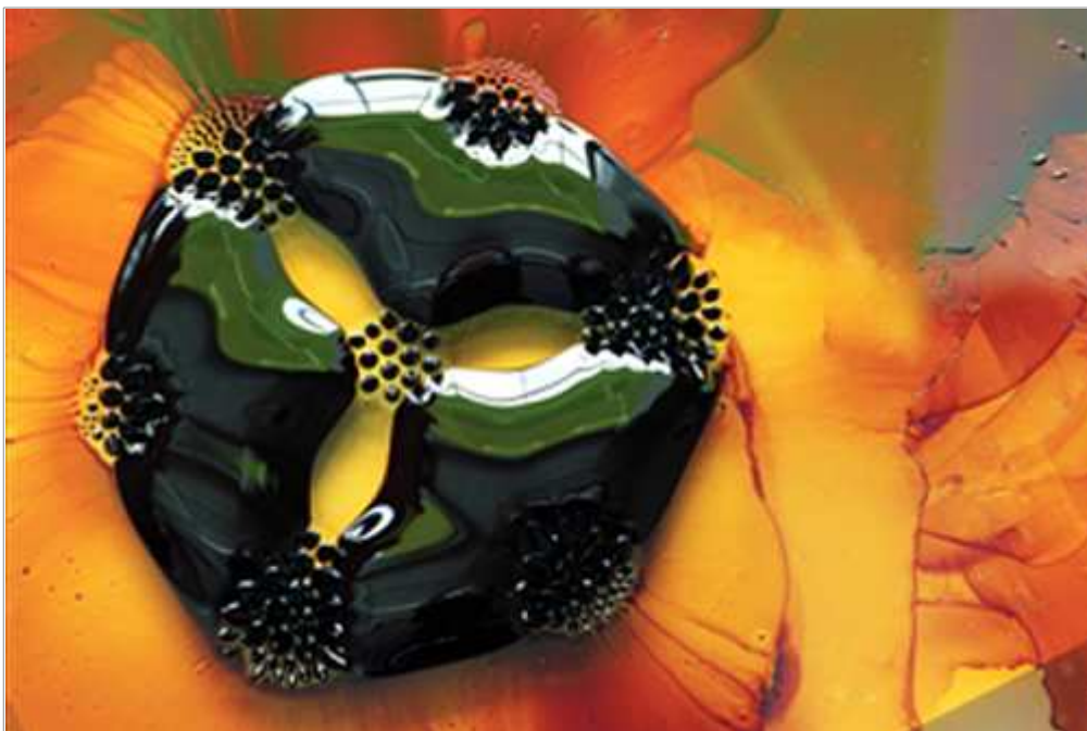
A 3-cm drop of ferrofluid on a glass slide. A slip of yellow paper sits below the slide and a set of seven small circular magnets under the paper affects the form of the drop
